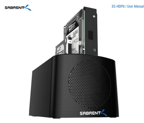
With a Sabrent EC-HDFN SATA Docking Station you can easily Hot-Swap 2.5"/3.5" SATA Hard Drives when connected to your Desktop or Notebook. As a Standalone Duplicator Dock it can be used to duplicate/clone an existing hard drive without connecting to a computer.
